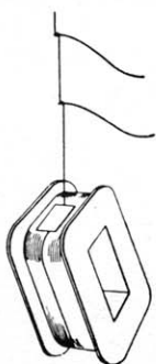
Fig. 1. Two leads twisted at each end of the cleared section of wire.
