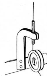
Fig. 3. Cotton sleeving held by clip.
